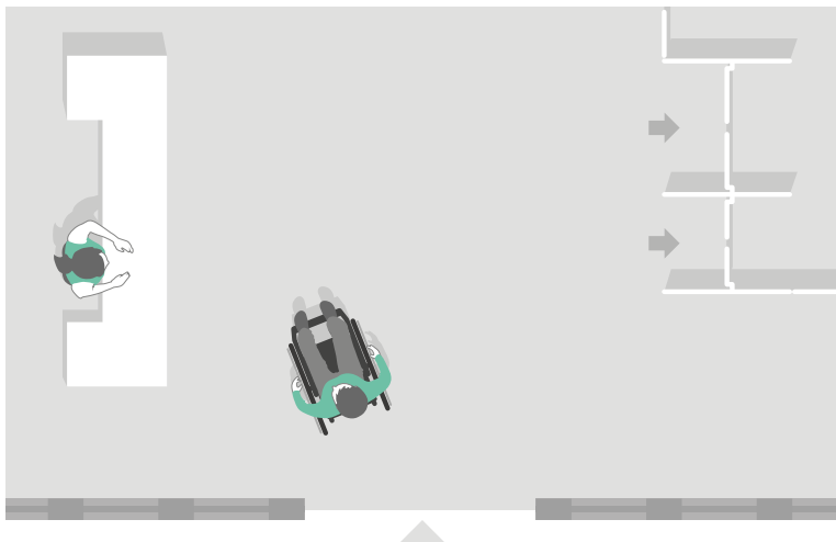
Example of circulation system in the building lobby - reception desk near the entrance, clear separation of visitor and employee traffic.
