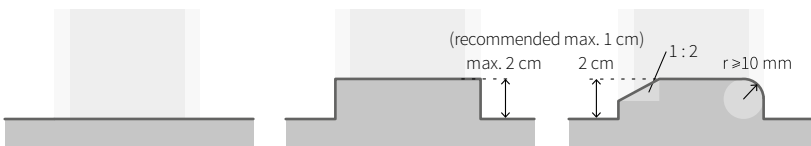
Cross-section through threshold: no threshold (recommended solution), threshold up to 2 cm, 2 cm threshold with min. 10 mm on one side and chamfered min. 1 : 2 on the other side.
