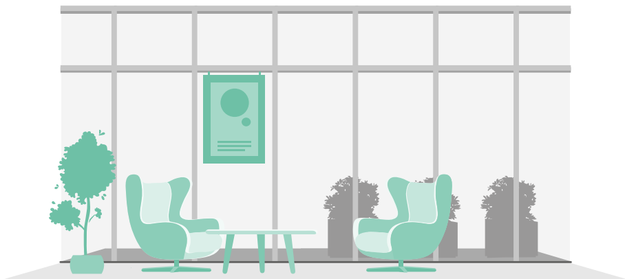
Furniture restricts access to the wall – marking is not necessary.
