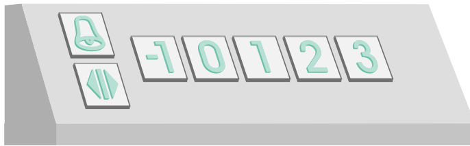
Inclined control panel to make it easier to hold the button while using the lift.
