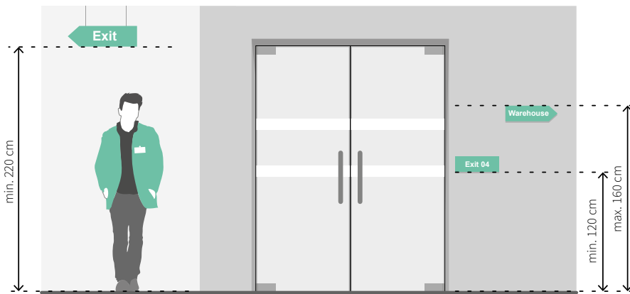
Installation height of information boards
